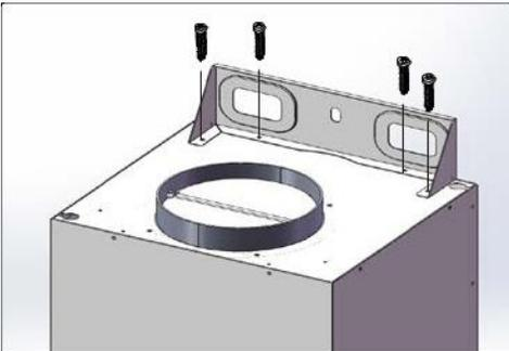
2. When attaching the appliance, ensure that it engages firmly with the brackets.
