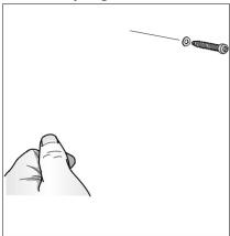
For the various installations use screws and screw anchors suited to the type of wall (e.g. reinforced concrete, plasterboard, etc.). If the screws and screw anchors are provided with the product, kindly check the screws are suitable for the type of wall in which the hood is to be fixed.
